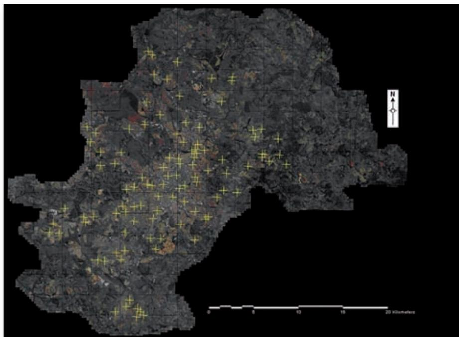
Figure 10 – Distribution of the independent geodetic points for the error and accuracy check.
