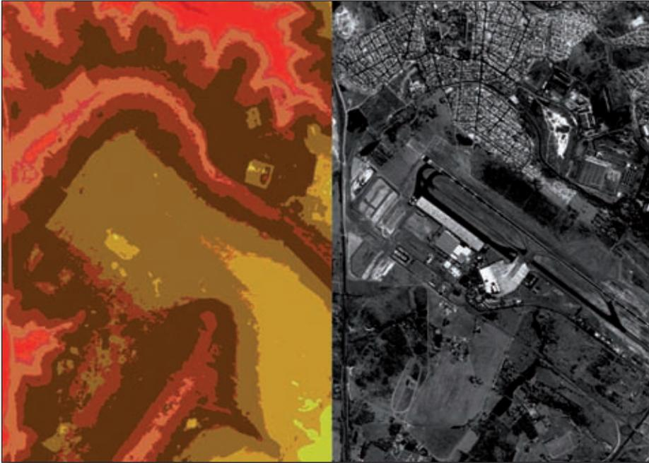
Figure 2 – Fragment of the DTM over the Viracopos International Airport (left) and correspondent WV-1 image (right).
