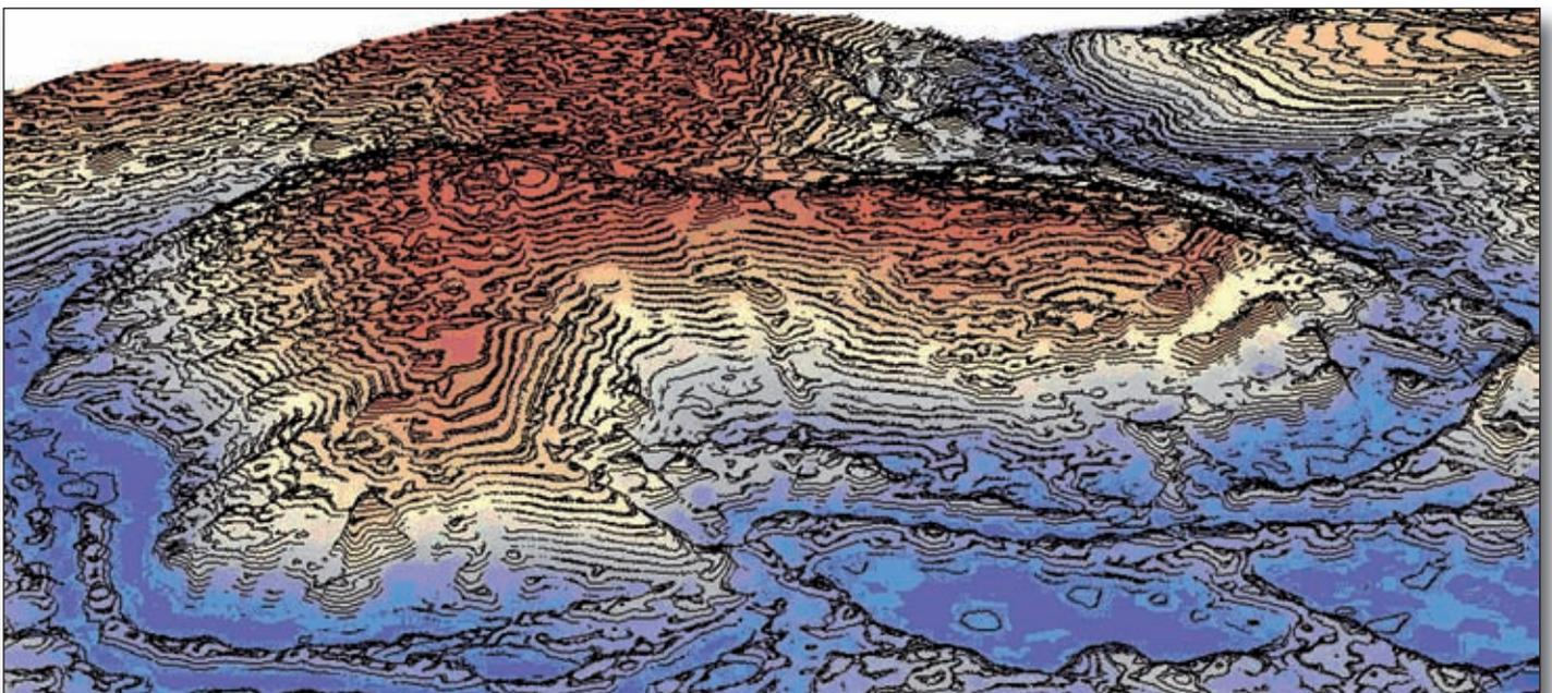
Figure 3 – 3D fragment of the DTM with contour lines.
